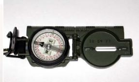
When using a Magnetic Compass, you have to remember to not have any rings, bracelets or other metal near it which could be slightly magnetized.
